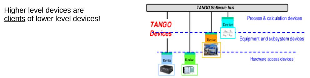
Figure 1 : The software bus view of devices
