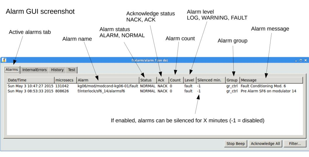
All the configuration is kept in the Alarm device server Properties or in the alarm database All the logic is maintained by the alarm device server, no logic in the GUI
